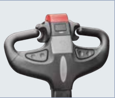
The ergonomic tiller head allows for easy operation with one hand
