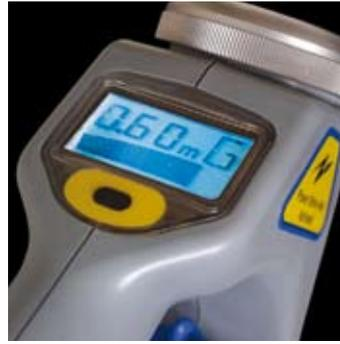
In the G mode the C.A.T³ detects a tone radiated by the Genny+ to a buried conductor.
