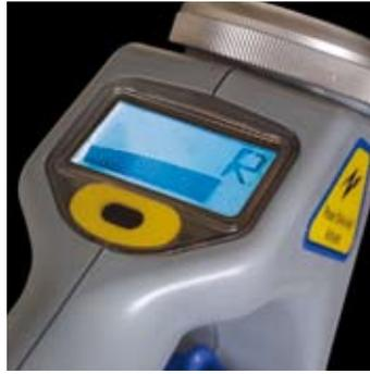
In the R mode the C.A.T³ detects VLF radio signals re-radiated by buried metallic pipes and cables.
