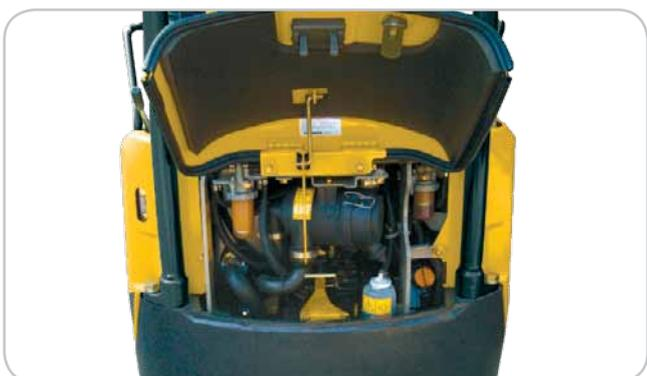
> Large rear bonnet allowing access to all engine components and hydraulic pumps.
