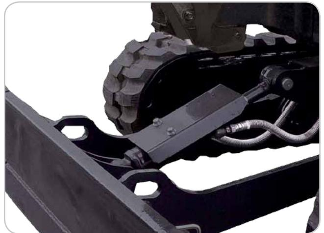
> The blade hydraulic cylinder is covered by a protective shield.
