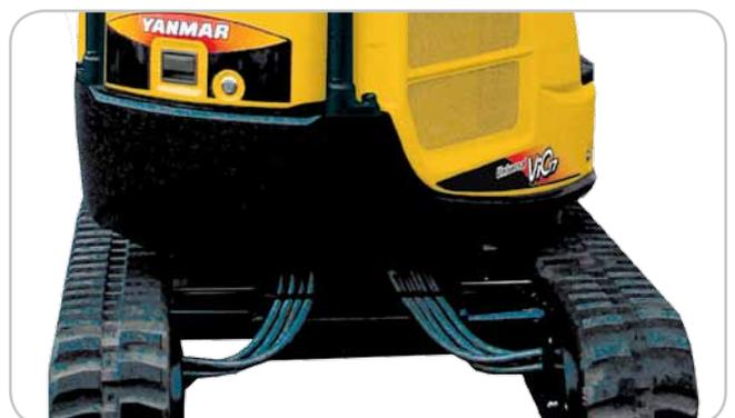
> Layout of the counterweight designed to protect the side panels against any possible shocks.
