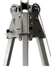
The head is made of **aluminum** and has 3 ball-bearing rollers for guiding the work rope on rescue or lifting devices
