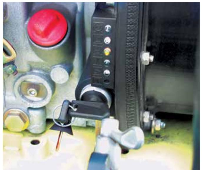
Elektric starter (option on APR 3020 Hatz Diesel)
