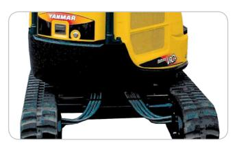
> Layout of the counterweight designed to protect the side panels against any possible shocks.
