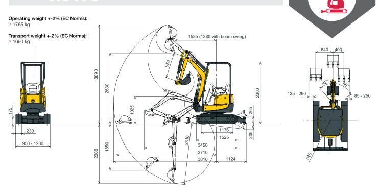
Subject to any technical modifications. Dimensions given in mm with standard Yanmar bucket.
