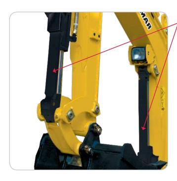
Bucket, arm, boom and blade cylinders completely protected (rod and cylinder) by highly elastic steel plates to resist any possible shocks.
